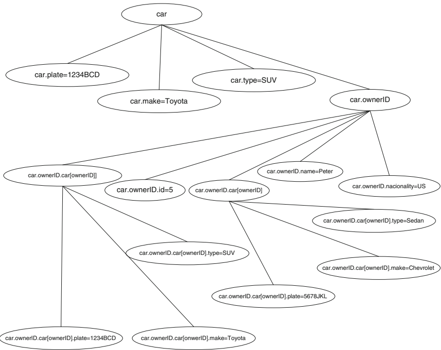
Fig. 8 Object-based tree derived from the multirelational database in Fig. 5 using car as the target relation
